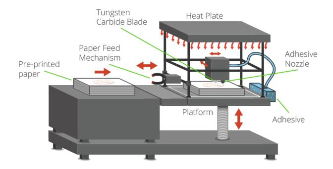
SDL is a proprietary 3D printing process developed and manufactured by Mcor Technologies. There is a temptation to compare this process with the Laminated Object Manufacturing (LOM) process developed by Helisys in the 1990's due to similarities in layering and shaping paper to form the final part. However, that is where any similarity ends.
